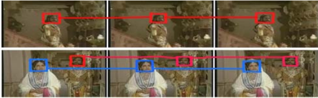
Figure 1: Top: a window consisting of frames 20000,20001,20002, Bottom: another window- with frames 21000,21001,21002. The detections are linked on spatio-temporal basis to form tracklets. One person (marked with red) occurs in both windows, the other (marked with blue) occurs only in the second. The two red tracklets should be associated though they are from non-contiguous windows
